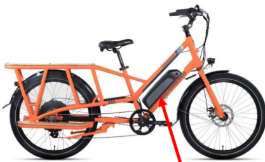
battery in frame
